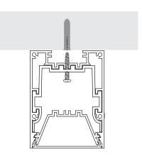
Drill holes in ceiling and fix with appropriate fasteners.
