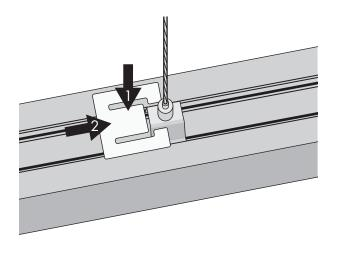
Fit packer clip as shown. Press down and then across until the arms are clipped in place.
