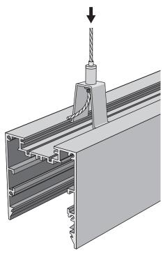
Install suspension wire to ceiling and thread into suspension clutch.
