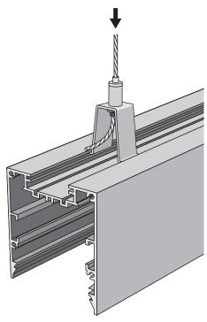
Install suspension wire to ceiling and thread intosuspension clutch. Ensure fittings are installed level.
