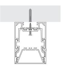
Drill holes in ceiling and fix with appropriate fasteners.
